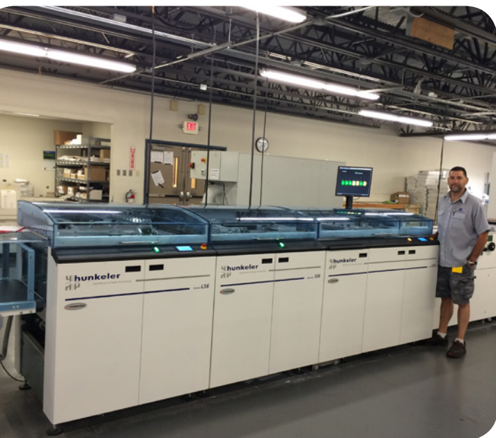
The Standard Hunkeler Roll-to-Stack solution, pictured here with Lead Operator Paul Vargas, runs inline with the Canon Océ ColorStream 3900 at Universal Wilde.
