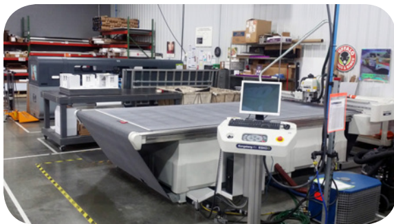
A key to wide format inkjet production is finishing. The Esko Kongsberg XN24 table was an easy decision.
